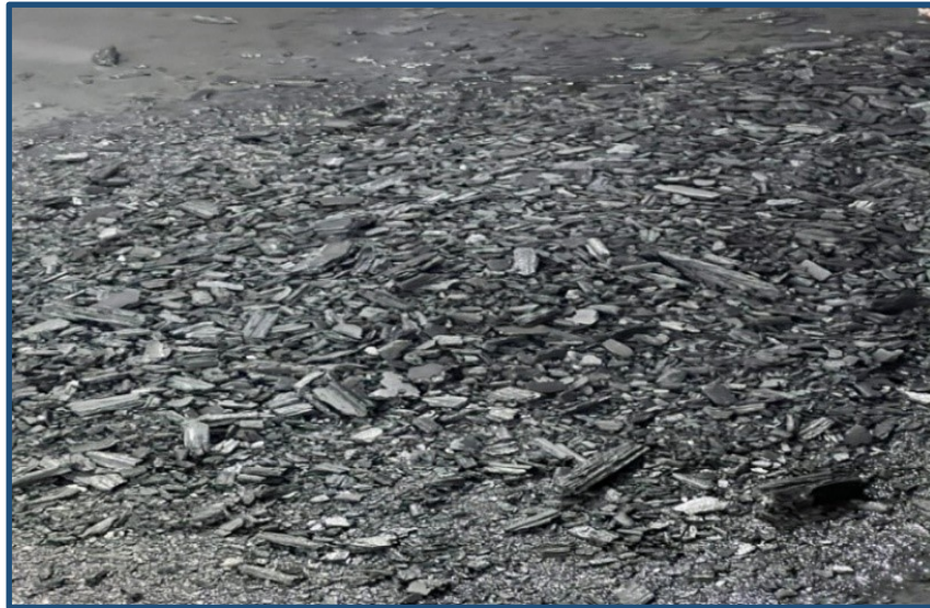
Figure 5. Hard grey scales recovered after hydro-jetting.
